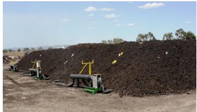
Photo 4: 1,500m 3 batch with temperature probes
